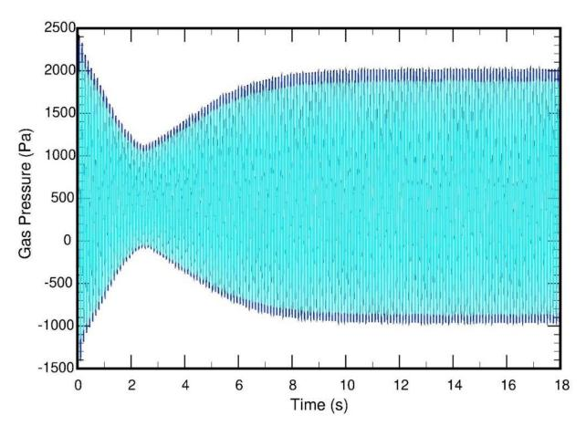
Figure 1 – The pressure response of a simulated Sondhauss tube illustrating an initial transient that decays and later amplifies to the steady sustained oscillation [1]
