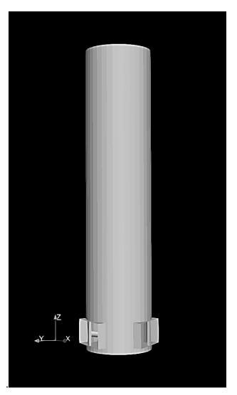
Figure 3 – The flare used in this thermoacoustic simulation has a height of 15 meters with a diameter of 3 meters and louver openings at bottom for air inlets
