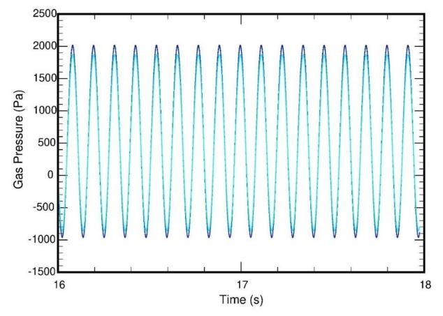
Figure 2 - Expanded time scale of the steady pressure waves allowed frequency to be determined [1]
