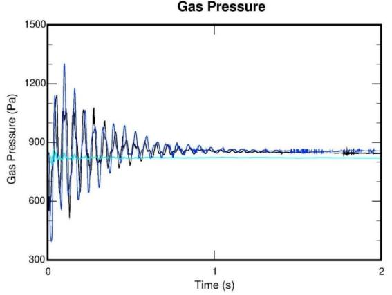
Figure 6 - The pressure waves within the flare caused by the sudden onset of flow decay rapidly a sound free condition under no-wind conditions
