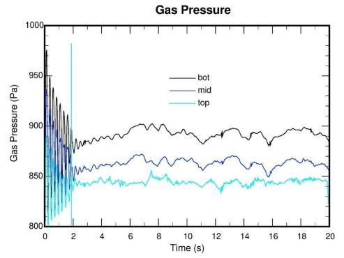
Figure 7 - The gas pressure at various elevations with a cross wind showing low amplitude persistent sound waves within the stack
